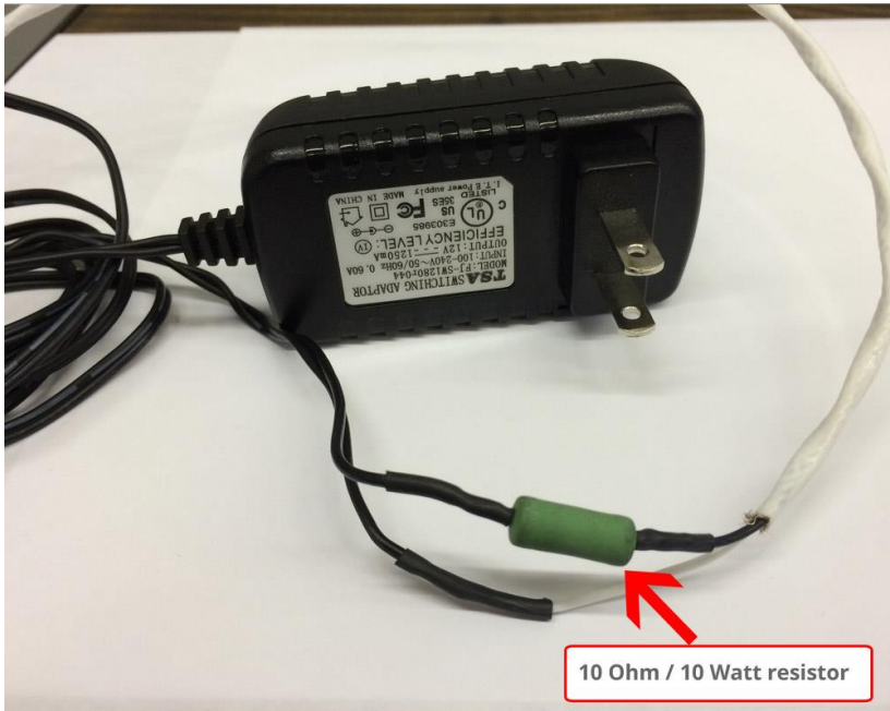
Image 6 – Power adapter with resistor is necessary if you do not have a doorbell chime
