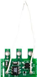
Image 4 – Digital doorbell adapter with 2 white wires
